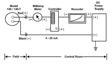
The 4-20 mA vibration transmitter output can be displayed with the milliampere meter. Other measurement instruments can be connected in the loop also. For example, a single 140 can support multiple instruments such as digital meters, process controllers, DCS, data loggers, recorders and PLCs.
